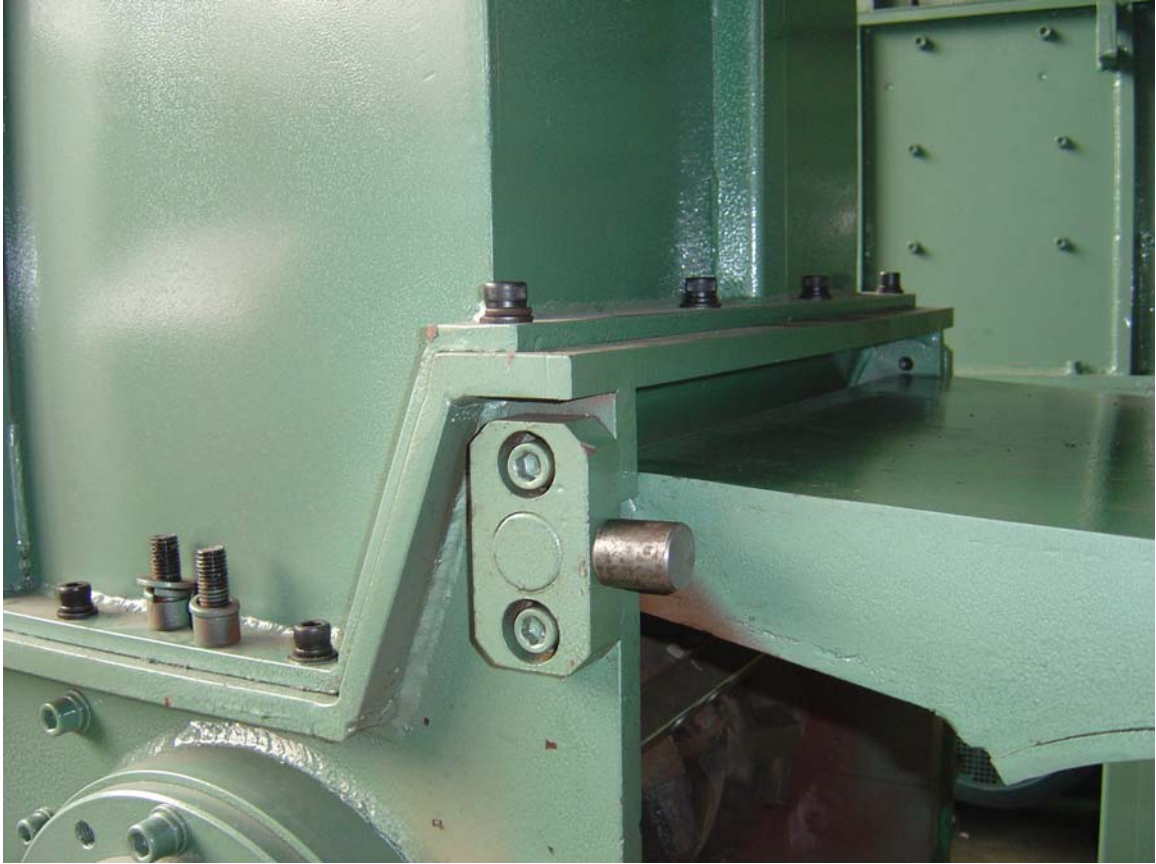
This picture shows the door pin in place holding up the screen assembly door.
