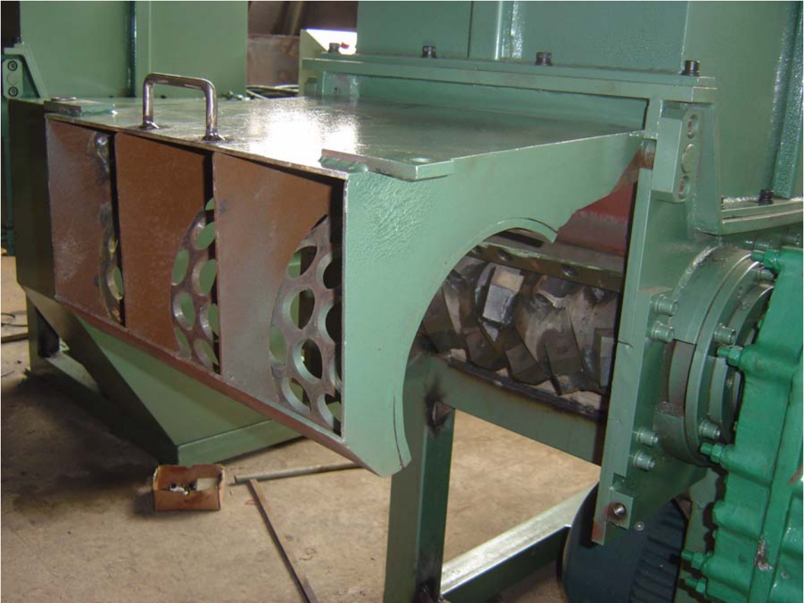
This is a picture of the Screen Assembly which rotates out of position to allow for maintenance of the Rotor and the Bed Knives and changout of the Sizing Screen.
