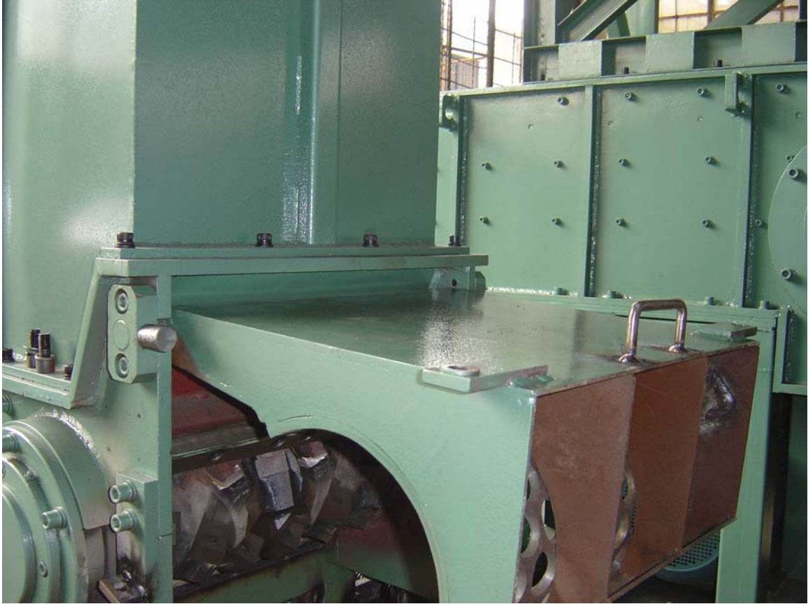
This is another picture of the screen door assembly in its maintenance position.
